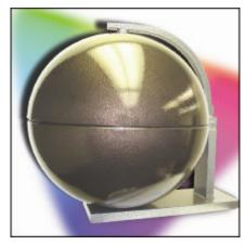
The **StellarSphere IS12** is a 12" integrating sphere that opens to allows for simple internal mounting of devices for light measurement such as discrete LEDs, arrays, and more. A tungsten halogen bulb and data file are included for system calibration using the SpectraWiz® radiometer software.
