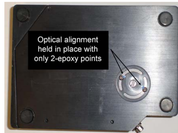
Figure 1: View of the bottom of an OOI HR4000 showing the rotating optical bench held in place with epoxy (blue).
